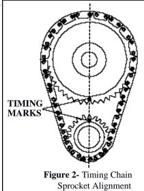
as recommended by factory specifications. See Figure 2. When using Performer-Plus Timing Chain and Gear Sets (7800 series) with Edelbrock cam and lifter kits, straight up timing alignment is achieved. If any other timing gear set is used, it is necessary to check cam position for correct timing alignment. This requires indexing the camshaft with a degree wheel to verify timing alignment. O.E.M. or non-Edelbrock timing gear sets are not recommended for use with Edelbrock camshafts.
