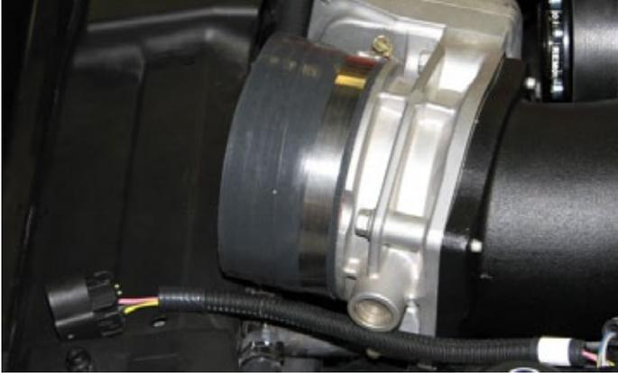
222. Install the grommet supplied in Bag #5 into the new air inlet tube.
