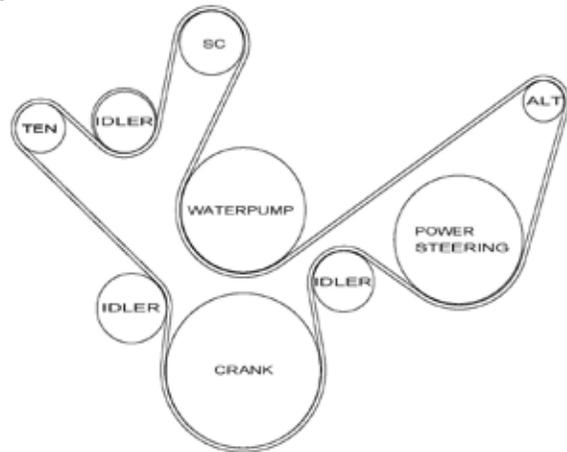
217. Use a breaker bar and a 16mm socket to push the tensioner enough to get the belt on, then double check the routing.
