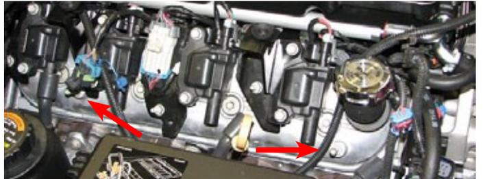
209. Remove the grommets from the stock coil covers.
