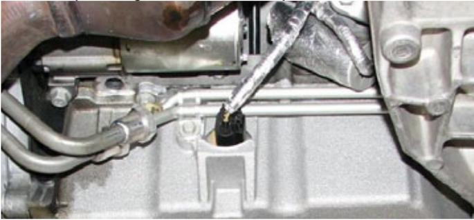
96. Use a 10mm socket to remove the starter support bracket bolt.
