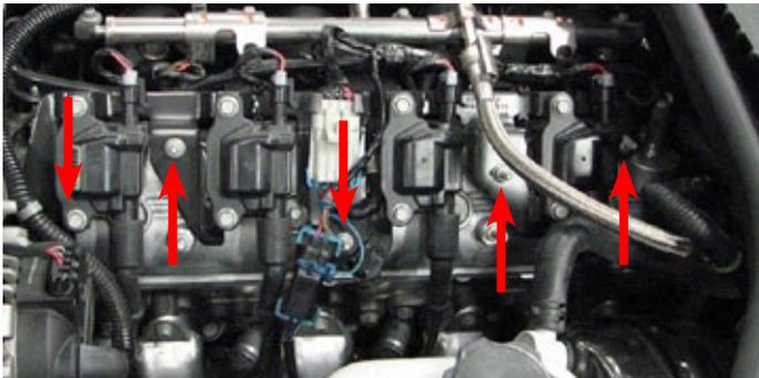
38. Use a fuel line removal tool to disconnect the fuel line from the rails using a shop rag to absorb excess fuel.
