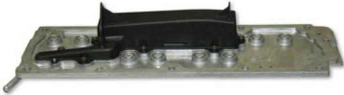
58. Apply anti-seize to the tapered surface beneath the heads of the countersunk bolts supplied in Bag #3 and install the valley plate with the stock perimeter gasket. Tighten the bolts from the center out with a 5mm allen tool then torque them to 18 ft-lbs in the same sequence.
