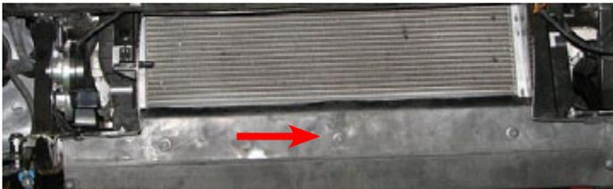
154. Disconnect horn electrical connector then use a 10mm socket to remove the bolt holding the horn bracket in place. Remove the horn assembly and set it aside.
