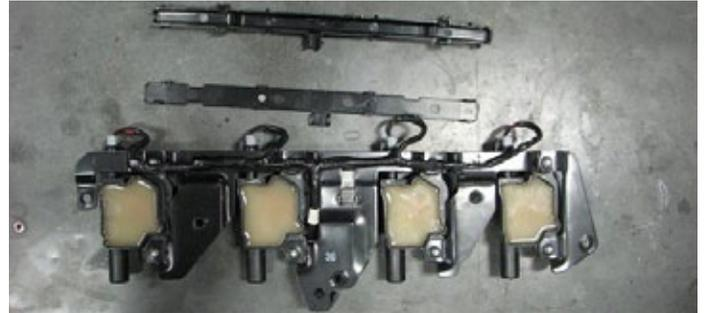
206. Tuck the fuel injector wiring harness and the EVAP Solenoid to Firewall Fitting Hose under driver side coil bracket then use a 10mm socket and the ten stock bolts to install both coil brackets on to the valve covers.
