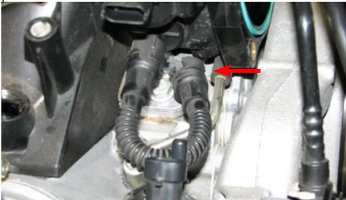
50. Remove the intake manifold and disconnect the small vacuum hose at the rear of the manifold next to the larger brake booster hose. Leave this hose connected to the firewall as it will be reused later.
