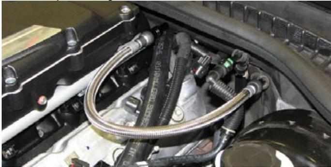
204. Connect fuel injector electrical connectors.
