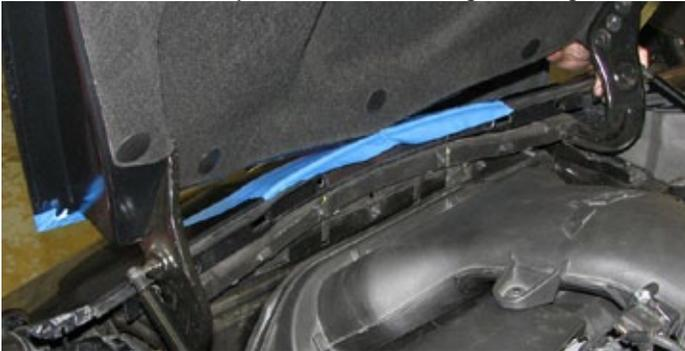
27. The sides of the fascia can be pulled away from the clips holding it in place, then down off the studs. The center section must be pulled up and over the nose section, and the whole assembly pulled straight off and set aside.
