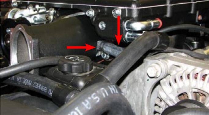
191. Use a 10mm universal socket with an extension bar to install the eight intake manifold bolts following the torque sequence below. Torque the bolts to 4 ft-lbs in the first pass, then to 7.5 ft-lbs in the second.
