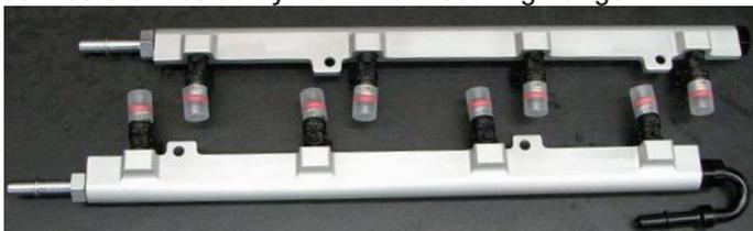
195. Apply O-ring lube to the sealing ring of the four supplied fuel rail fittings. Use a 3/4" wrench to install the two straight hose fittings on the radiator side of each fuel rail then install the plug in the firewall end of the passenger side fuel rail and the U-shaped fitting on the firewall end of the driver side rail. Orient the fitting close to the injector, leaving room for the injector connector.
