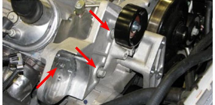
144. Use an 8mm allen tool to install the 45mm bolt supplied in Bag #1 that retains the tensioner bracket to the cylinder head and torque it to 37 ft-lbs.
