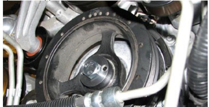
103. Use a 24 mm socket to install the supplied bolt and reamer guide to the end of the crank.
