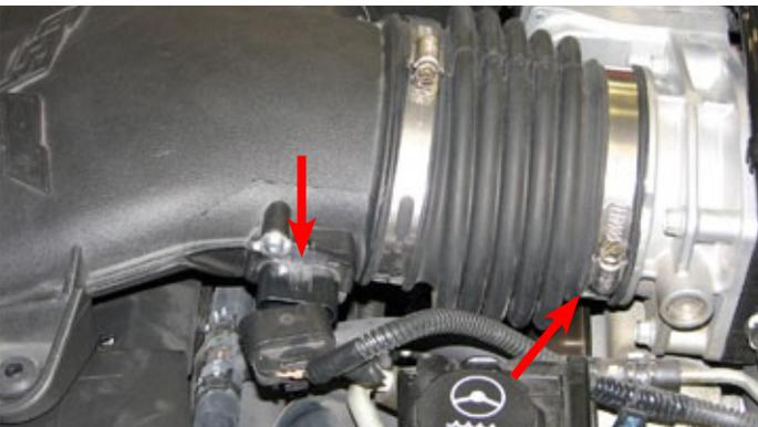
29. Use a flat head screwdriver to loosen the Throttle Body to inlet tube worm clamp.
