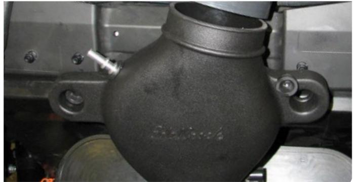
229. Slide the nose of the air inlet tube into the air filter then hold the grommets in place with a socket as you tilt the air inlet tube down into the silicone tube and onto the locator pins.
