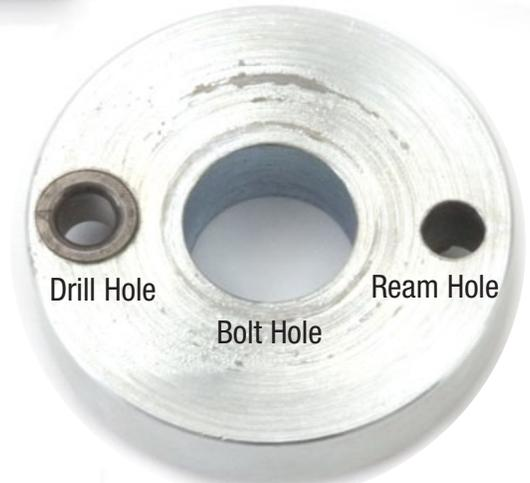
(1x) - Crank Pinning Drill Guide
