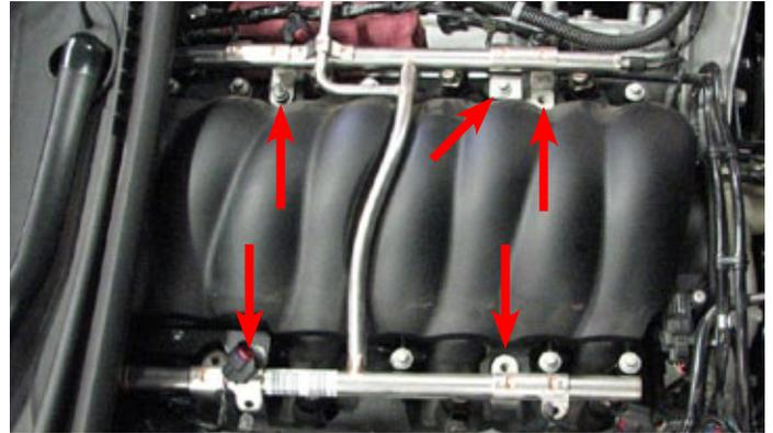
**NOTE:** You will also need to remove one 8mm manifold bolt and bracket before removing the fuel rails.
