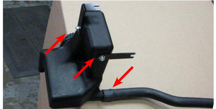
177. Use a 10mm socket to loosen rear hood hold down latch bolt on passenger side fender.
