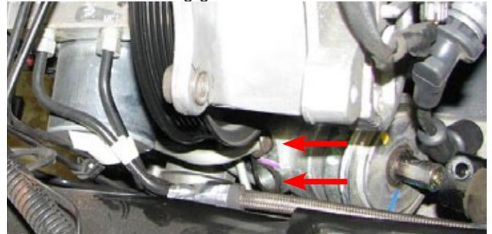
83. Use a 10mm socket to remove the bolts retaining the power steering line brackets or fluid cooler, if equipped.
