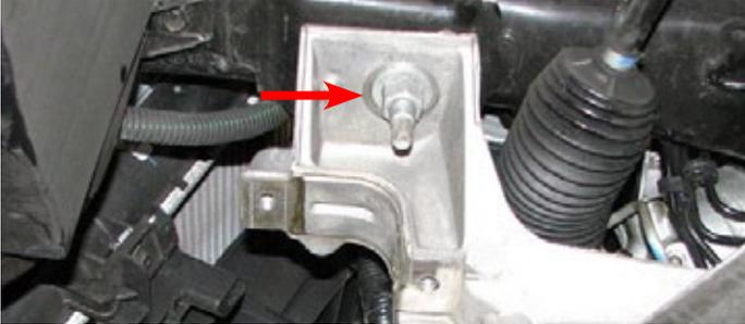
86. Disconnect the ride height sensor electrical connector from each side, if equipped.
