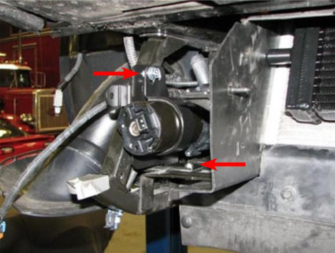
**NOTE:** There are two different water pump brackets: Version (1) requires the use of your OE horn bracket. Version (2) has an integrated horn bracket. You should have received one of the two brackets; If your supercharger kit includes bracket version (2), you may disregard Step 161.
