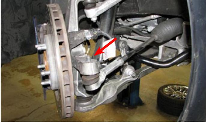
78. Use GM Ball Joint Separator #J 42188 to separate the steering knuckle from the tie rod ball stud then remove the tool and the nut. Use this procedure for both sides.
