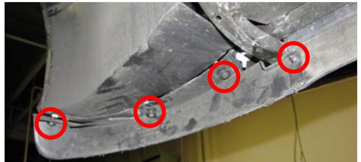
24. Remove the five 7mm and two 10mm nuts retaining the fascia from below.
