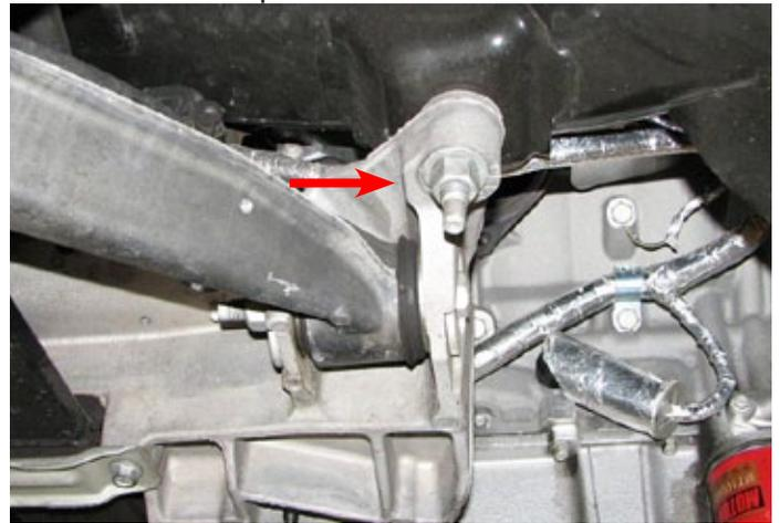
93. Insert a pry bar between the frame and front driver side cradle mount.
