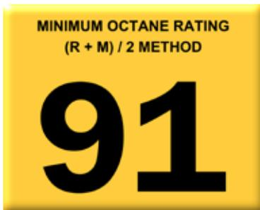
***91 octane or higher gasoline is required at all times. If your vehicle has been filled with anything less, it must be run until almost dry and refilled with 91 or higher octane gasoline twice prior to installation.***
