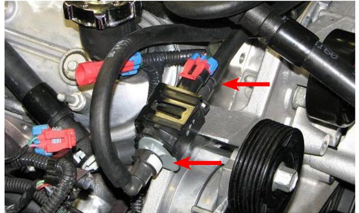
197. Apply O-ring lube to the lower seals of each of the fuel injectors.
