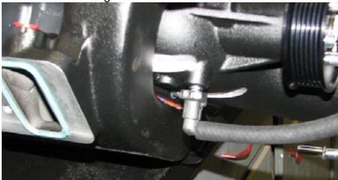
187. Clear engine valley of any hoses, wires, tools, etc. Lay the intercooler-to-reservoir tank hose in the engine bay, routed along the firewall behind the oil pressure sensor, and connect it to the intercooler reservoir inlet, securing the fitting with a hose clamp supplied in Bag #2.
