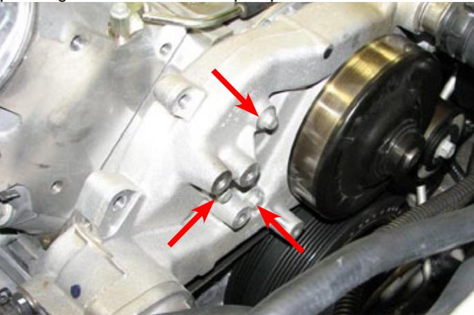
142. Use a 6mm Allen tool and the three 90mm bolts supplied in Bag #1 to install the lower idler bracket on the water pump then torque them to 18 ft-lbs.
