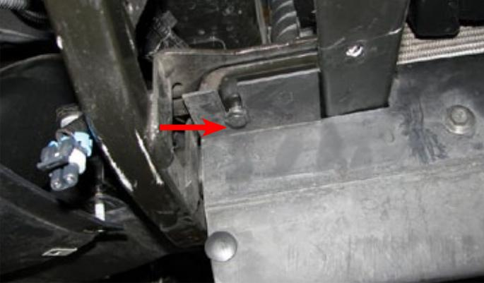
160. Use a 10mm socket to loosely install the water pump bracket using the stock horn bracket bolt on top and the bolt supplied in Bag #3 on the bottom.
