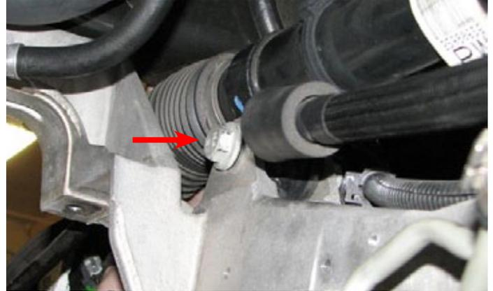
91. Remove the plastic clamp holding the power steering lines to the steering rack.
