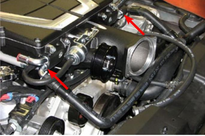
202. Attach one end of the supplied PCV hose to the 90° fitting below the air inlet on the supercharger. Route the other end of the PCV hose to the tube extending from the valley plate and attach
