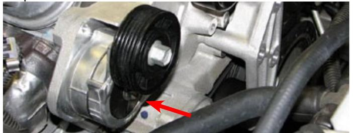
147. Use a 12mm socket and a 20mm bolt supplied in Bag #1 to mount the EVAP purge solenoid on the back of the new tensioner bracket.
