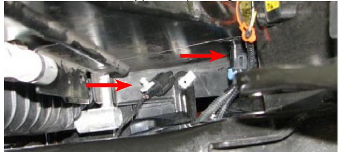
70. Reach up from below the car to remove the two remaining body pins retaining the front radiator shroud then remove the shroud by pulling it down and out.
