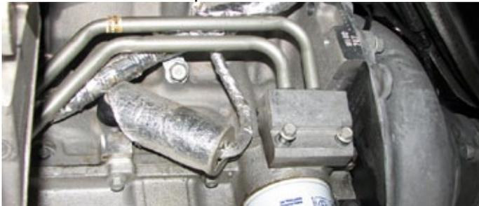
110. Use a 10mm socket to remove the two center oil pan rail bolts.
