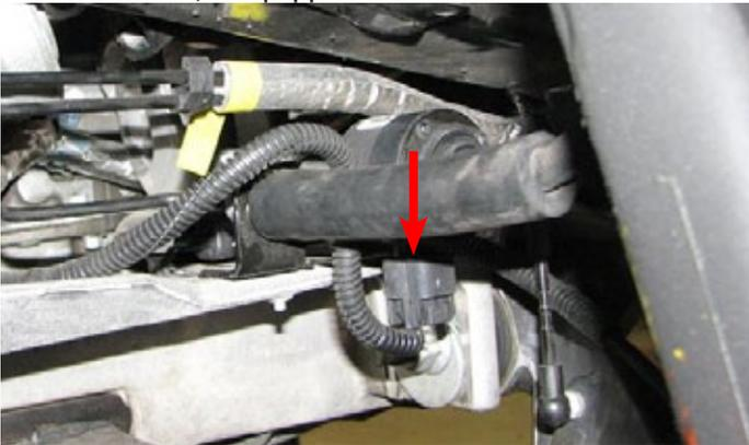
87. Use a 10mm socket to remove the driver side brake line bracket bolt.
