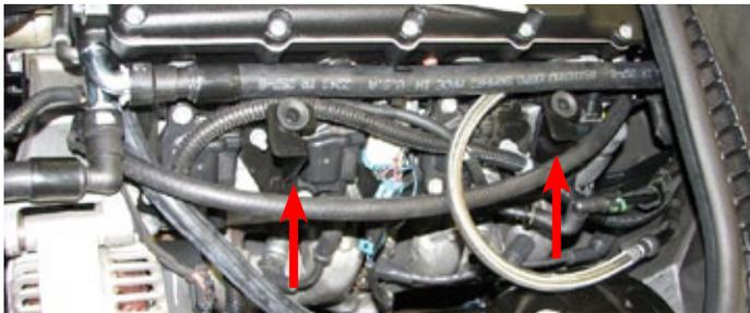
213. Tuck the wire harness tight against the fuel rails. Verify that nothing will be pinched or damaged when the coil covers are installed.
