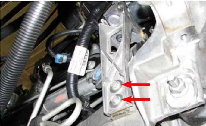
90. Use an 18mm socket to remove the two steering rack nuts and bolts.
