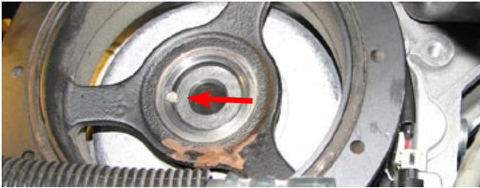
106. Install the supplied GM crank bolt into the crank and torque it to 37 ft-lbs, then rotate it an additional 140°
