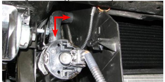
170. Lower the heat exchanger hose assembly along the driver side of the radiator shroud.
