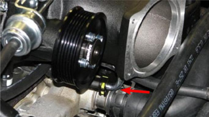
203. Install the supplied fuel line from the firewall fitting to the U-shaped fitting on the driver side fuel rail.
