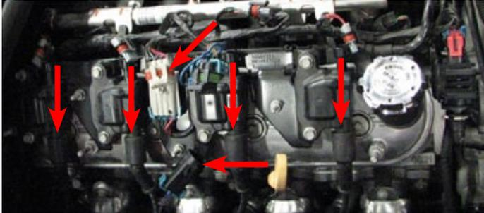
37. Use a 10mm socket to remove the five bolts retaining the coil bracket on each valve cover then remove both coil bracket assemblies.
