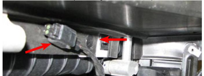
69. Disconnect the ambient air temperature sensor and remove the sensor clipped to passenger side of shroud.
