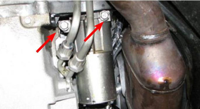
98. Disconnect electrical connector at top of starter, then use a 13mm socket to remove the nuts retaining power wires to the starter.
