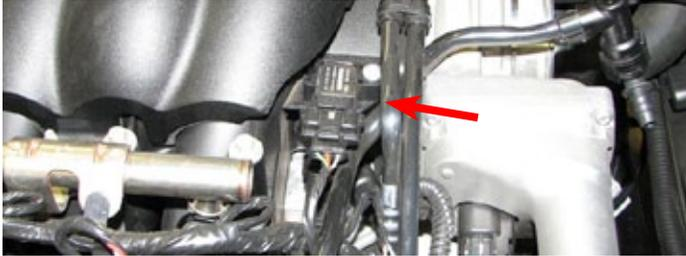
47. Disconnect the vacuum hose from the brake booster fitting; it will be removed with the manifold.
