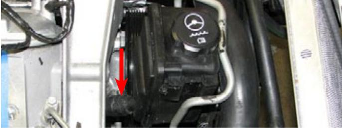
149. Slide the old bracket off the reservoir then install the supplied bracket using a 15mm socket and the stock bolts. Slide the power steering reservoir onto the new bracket and reattach the lower reservoir to pump hose.
