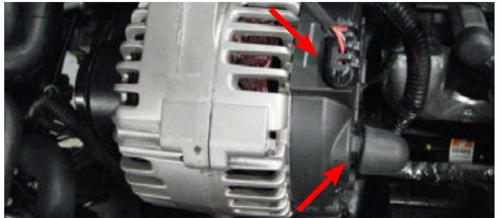
74. Use a 13mm socket to remove alternator power wire.
