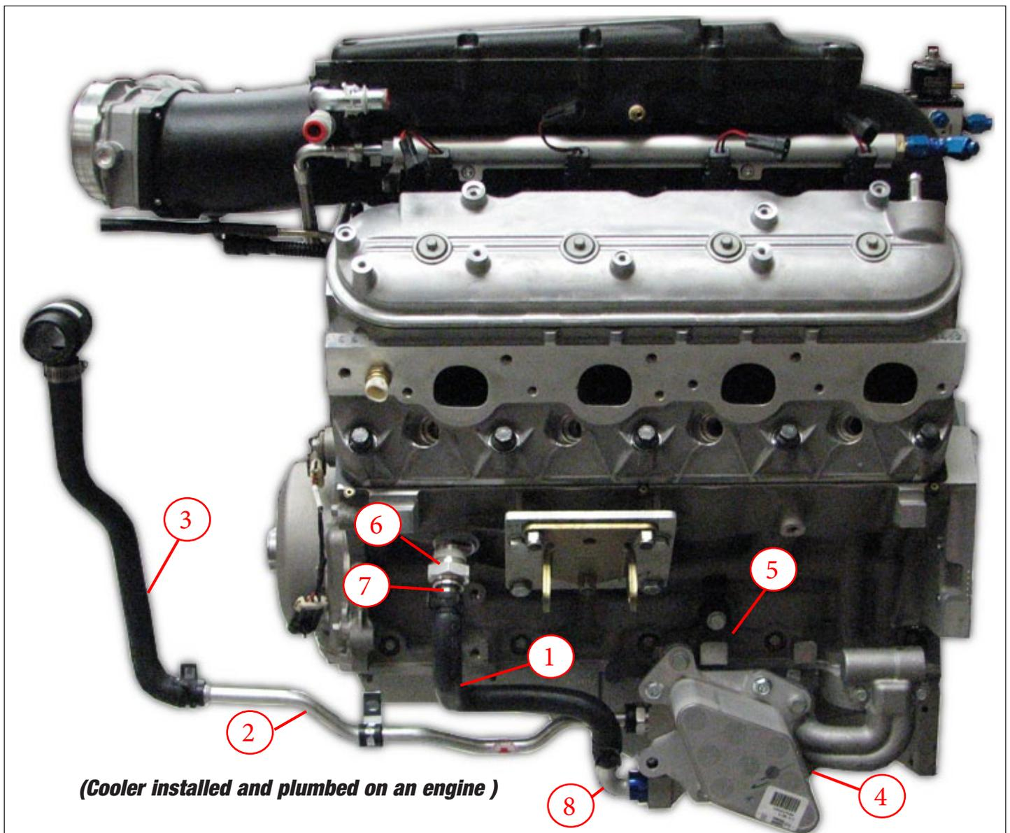
***(Cooler installed and plumbed on an engine )***
