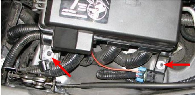
175. Use a 7mm socket to remove the fuse box bolt located in the passenger side fender well.
